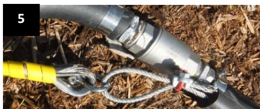
Check valve connection and secured steel cable eyelet from ballast.
