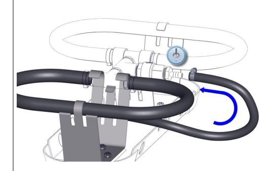
Step 9: Slide the provided hose clamp onto the SureSink tubing. Hose clamp size depends on the user's SureSink Size. Feed the weighted tubing over substrate connector leaving plenty of slack, make a generous loop and secure tubing to barbed fitting with the hose clamp.
