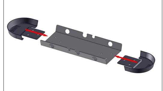
Step 5: Take the Substrate Connector Plate and the Substrate Edge Guards and slide the guards onto the connector as shown.
