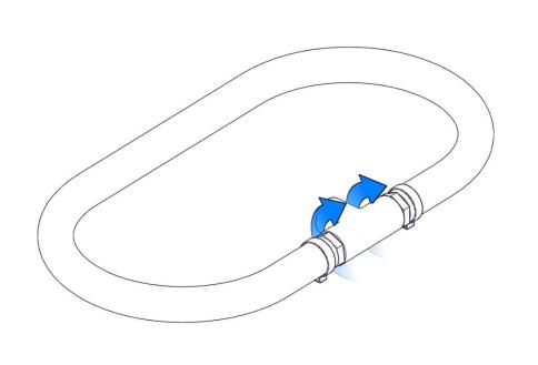
Step 1: After unpacking your box, the tubing assembly tee's open end will be turned towards the center of the loop. Twist the tee fitting so the open end will face away from the center of the tubing loop.
