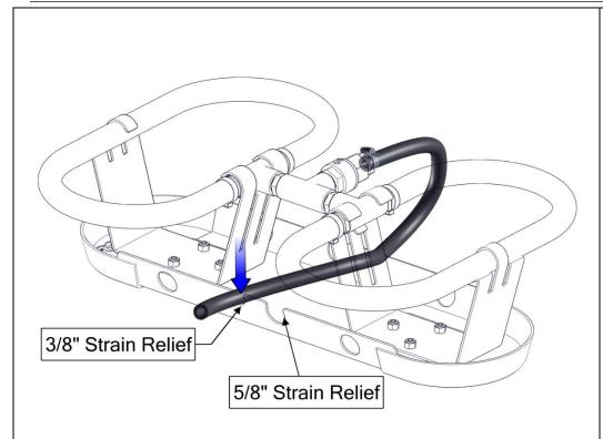
Step 10: Press weighted tubing into strain relief features on both sides of the connector plate, being sure tubing loop isn't too tight to cause strain on barbed fitting. Strain relief features are designed to accommodate both 3/8" and 5/8" SureSink tubing.
