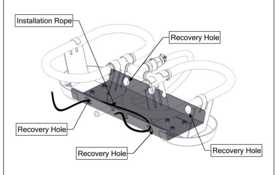
Optional Step: Once at the desired location thread a rope through two of the four recovery holes on the diffuser base. Pull through until the rope is at the midway point on the diffuser base.
