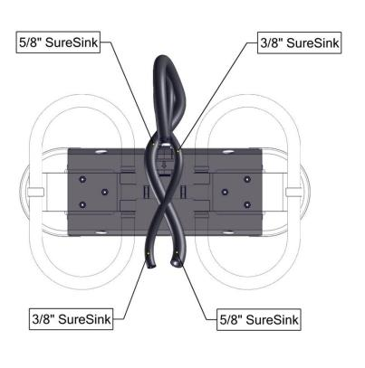
**Step 11:** The SureSink strain reliefs run diagonally through the substrate connector plate. Make sure to press the Sure Sink into both correctly sized holes before installing the unit.
