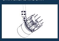
Adjustable angle and depth options. Uses a 1 in. (25 mm) nominal threaded or unthreaded pipe, customer supplied. Simple Swivel bracket allows unit to easily rotate and direct the flow of water.
