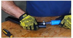
3- On the other end of the Bubble Tubing<sup>®</sup> insert a plug and secure it with a clamp.
