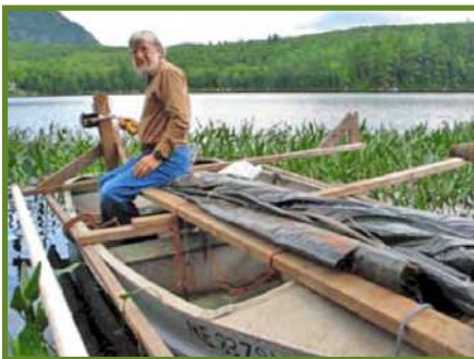
Jim Chandler with CLA's modified ATV winch mat-winder. This system, though somewhat finicky, was an improvement over the earlier bicycle crank-winder.
