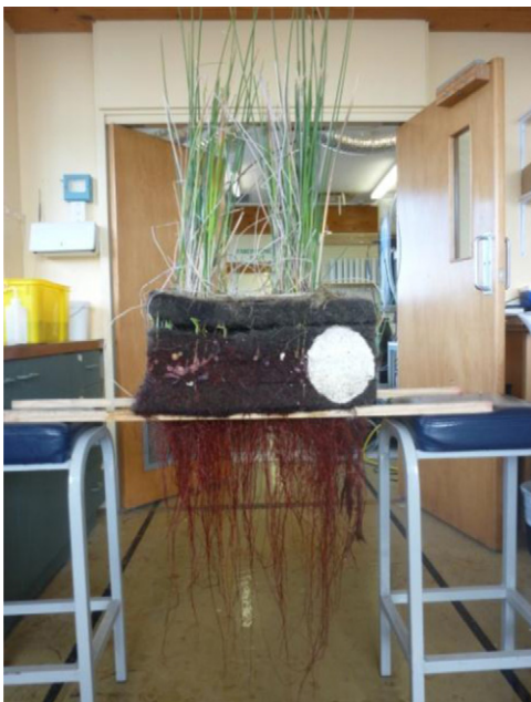
Fig. 2. Cut section of a FTW planted with Schoenoplectus tabernaemontani .
