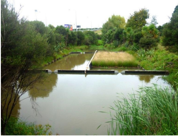
Fig. 1. FTW on the surface of a retention pond which is the experimental site of the present study – left: conventional (Control in this study) pond, right: FTW pond, foreground: inlet forebay.
