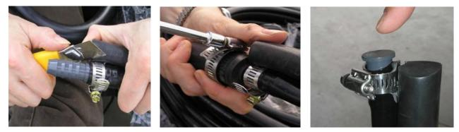
Make sure not to cut the air tube (superior part) when using an x-acto to make the slits at the end of the lines to install the clamps (see above pictures).
