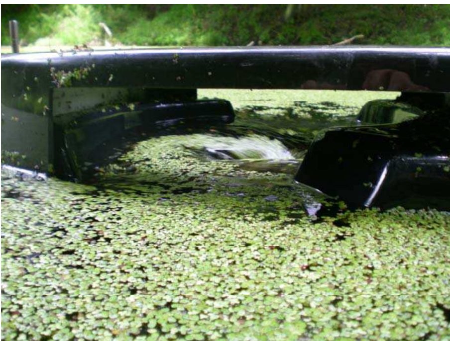
Figure 23 Optimal skim- ming depth. Note the water level entering the inlets. This level will be different (usually higher) when the System is not running.
