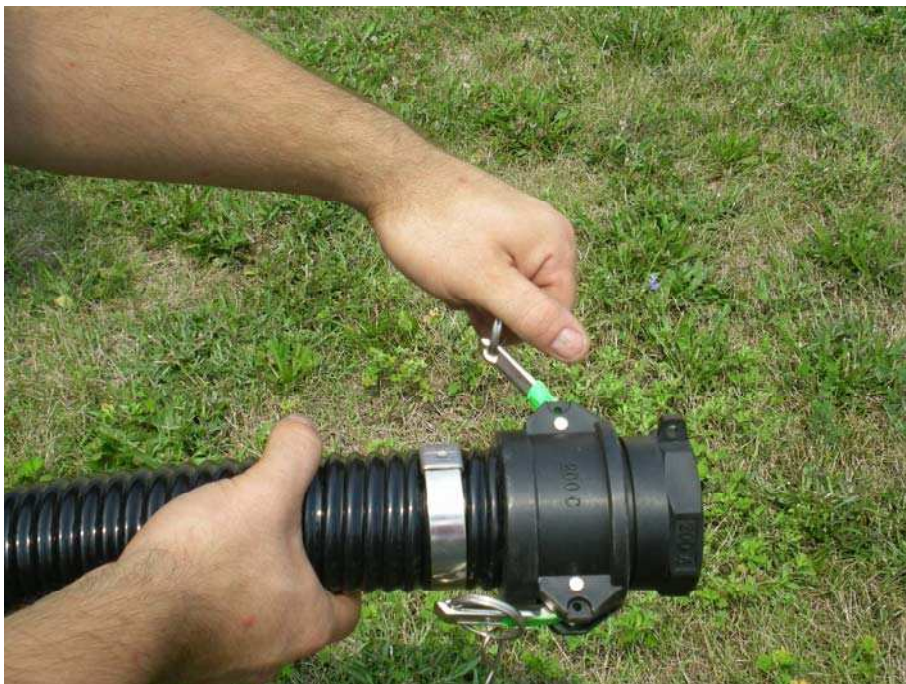
Figure 6 Removing the cam-lock quick connect fitting that shipped with your System.
