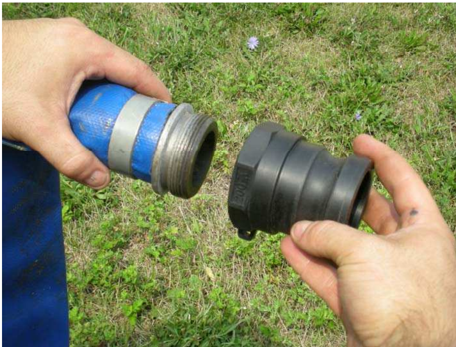
Figure 7 Screw the quick connect fitting on to your 2-inch hose.
