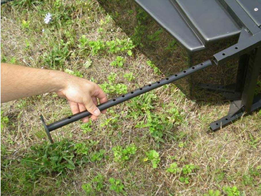
Figure 2 Inserting the adjustable legs into the filtration unit.
