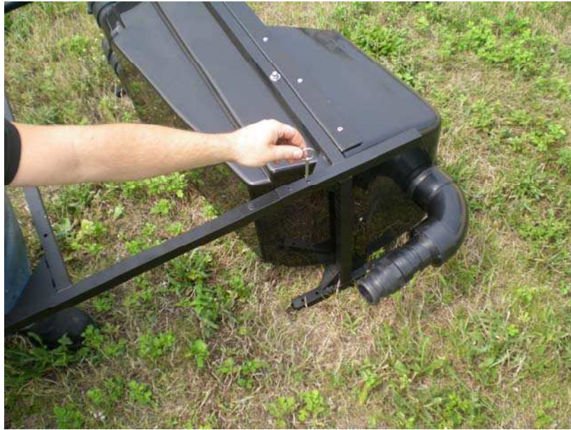
Figure 17A Locking the extension legs into the body of the filtration unit with pushpins.
