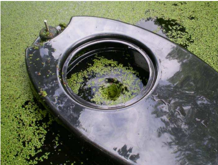
Figure 22 Proper vortex formation with correct skim- ming depth.
