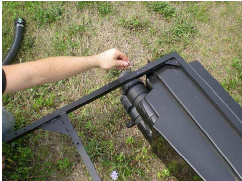
Figure 17B Locking the extension legs into the body of the filtration unit with pushpins.
