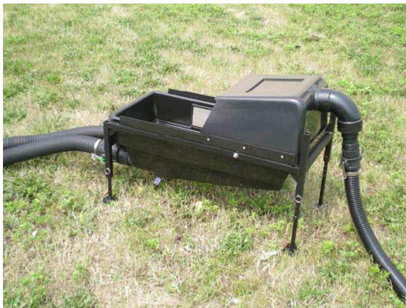
Figure 15 2 inch quick connect hose properly con- nected.
