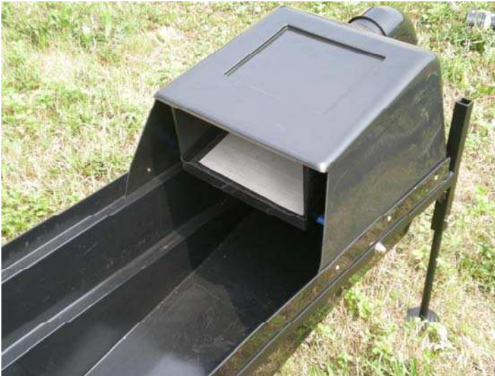
Figure 10 The correctly inserted primary filter.
