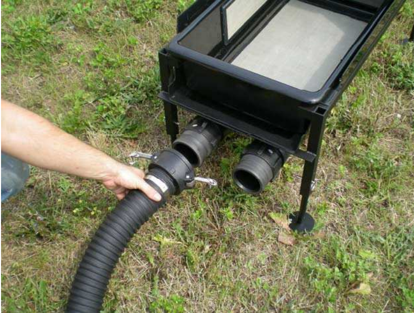
Figure 13 Connecting the 3 inch outlet hose.
