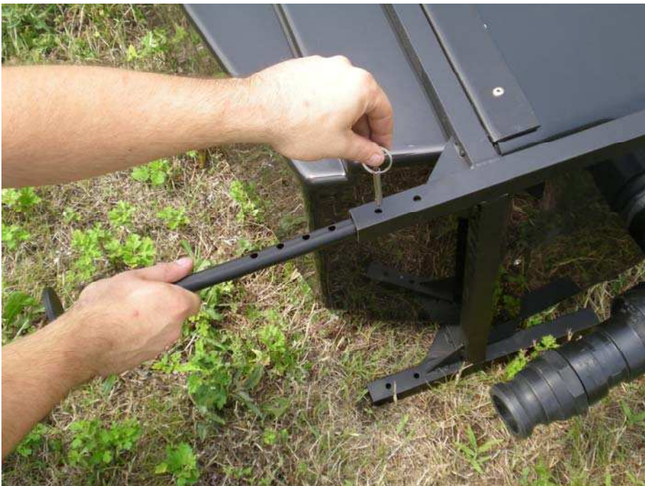
Figure 3 Locking the adjustable legs with a pushpin.
