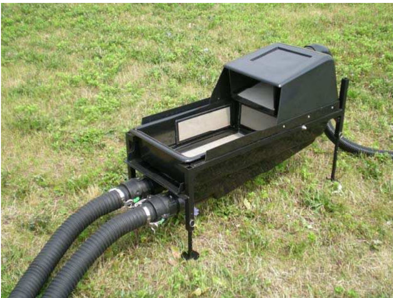
Figure 14 3 inch quick connect hoses properly con- nected.
