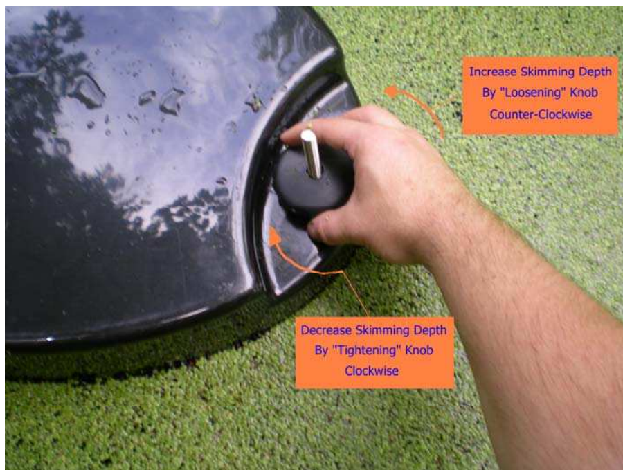
Figure 24 Adjusting the skimming depth adjustment knobs.
