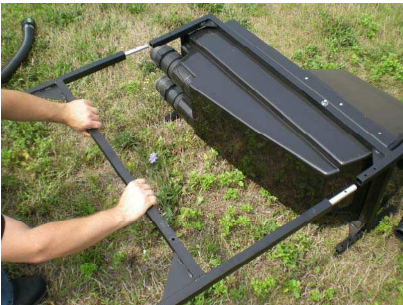
Figure 16 Inserting the extension legs into the body of the filtration unit.
