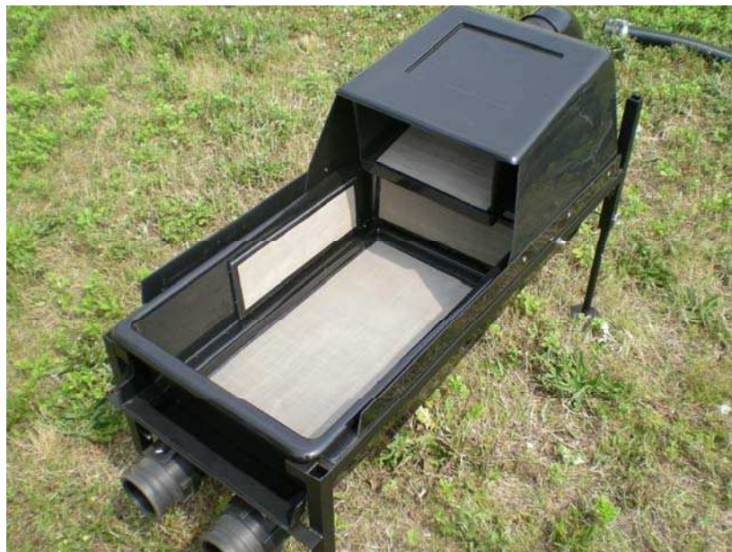
Figure 12 The collection box correctly inserted.
