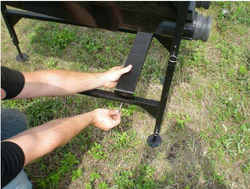
Figure 18 Attaching the extension leg cross members and securing with pushpins.
