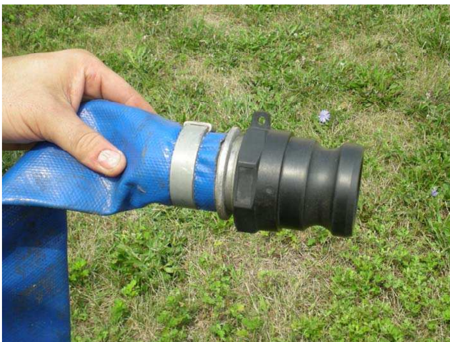
Figure 8 Quick connect fitting secured to your 2 inch hose.
