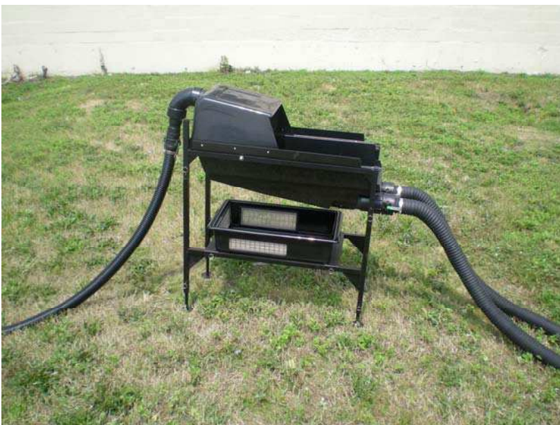
Figure 19 Extension leg assembly completed and ready for installation of the collection chute.
