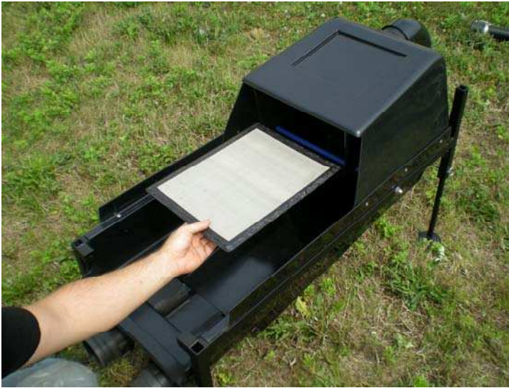
Figure 9 Inserting the primary filter.
