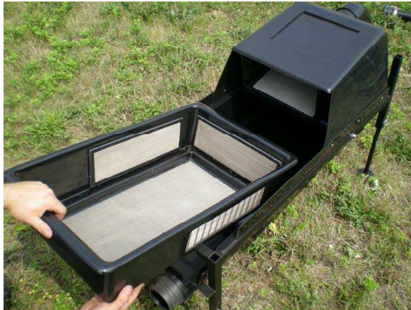
Figure 11 Inserting the collection box.
