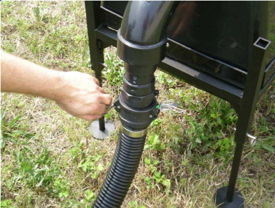
Figure 5 Locking the 2 inch cam-lock connector in place.
